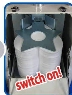
Finally, put the star weight attached to the WD-7C and close the lid of the device.
